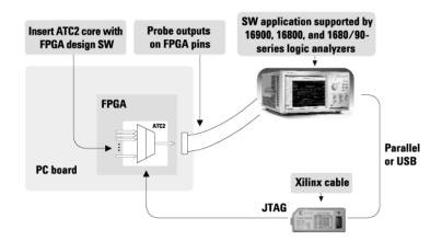
Create a time saving FPGA measurement system. Insert an ATC2 (Agilent Trace Core) core into your FPGA design. With the application running on your logic analyzer via JTAG you control which group of internal signals to measure.
