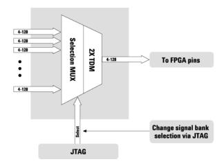
Access 64 internal signals for each debug pin. Select cores with 1, 2, 4, 8, 16, or 32 signal banks. Signal banks all have identical width (4 to 128 signals wide) determined by the number of pins you devote for debug. Each pin provides sequential access to 1 signal on every input bank. Using an optional 2X time division compression in state mode, each pin can simultaneously access 2 signals per bank.
